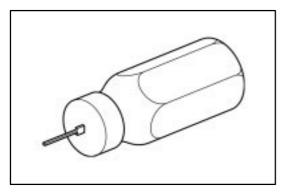
Preparation of the SST to release the 0.64 connector terminal. SST 09991-00500
